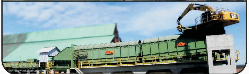
Debarking is done through the friction between processing logs, as well the abradars' action, which takes the bark off the logs and forwards the material along the debarker.
