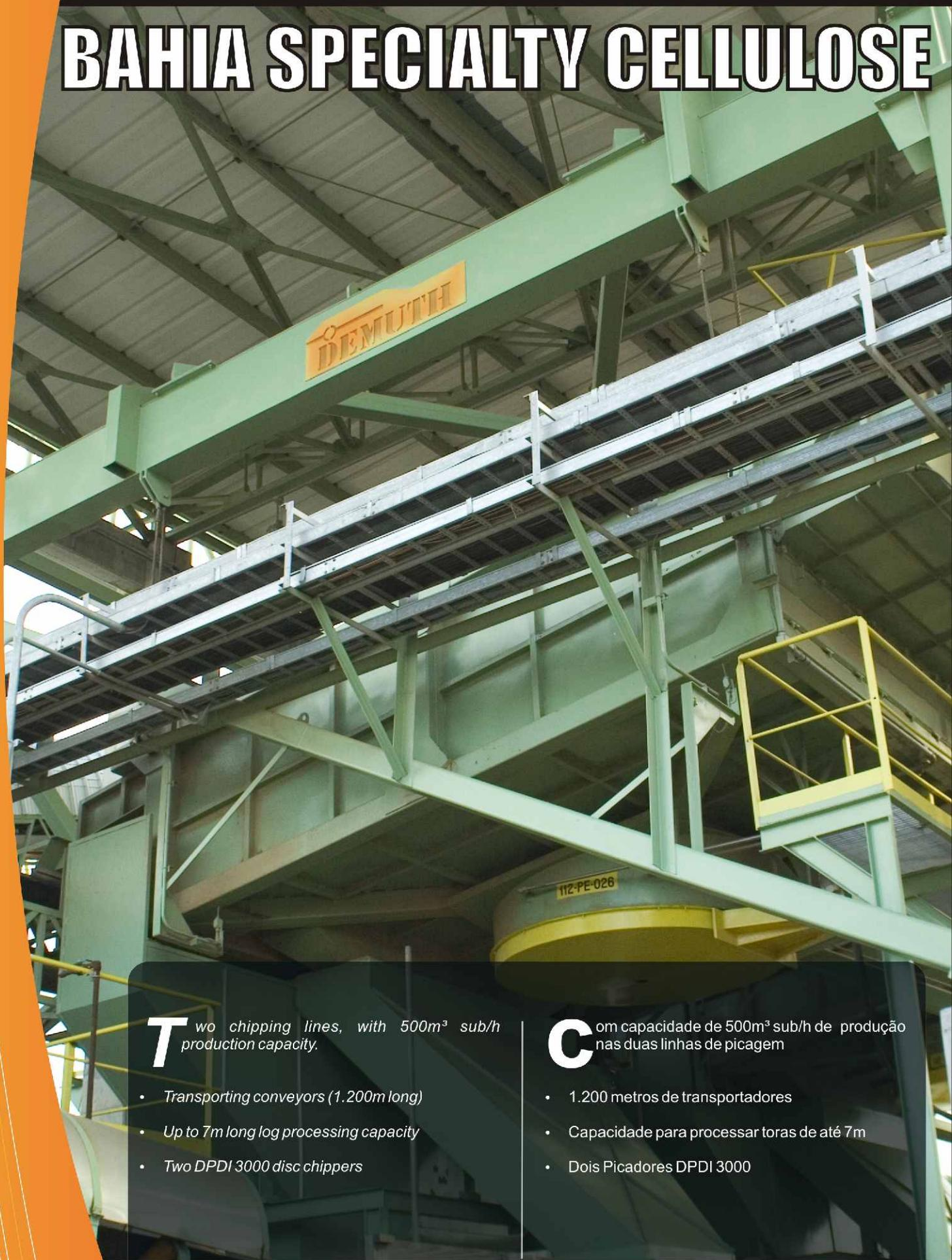
**T**wo chipping lines, with 500m<sup>3</sup> sub/h production capacity.
