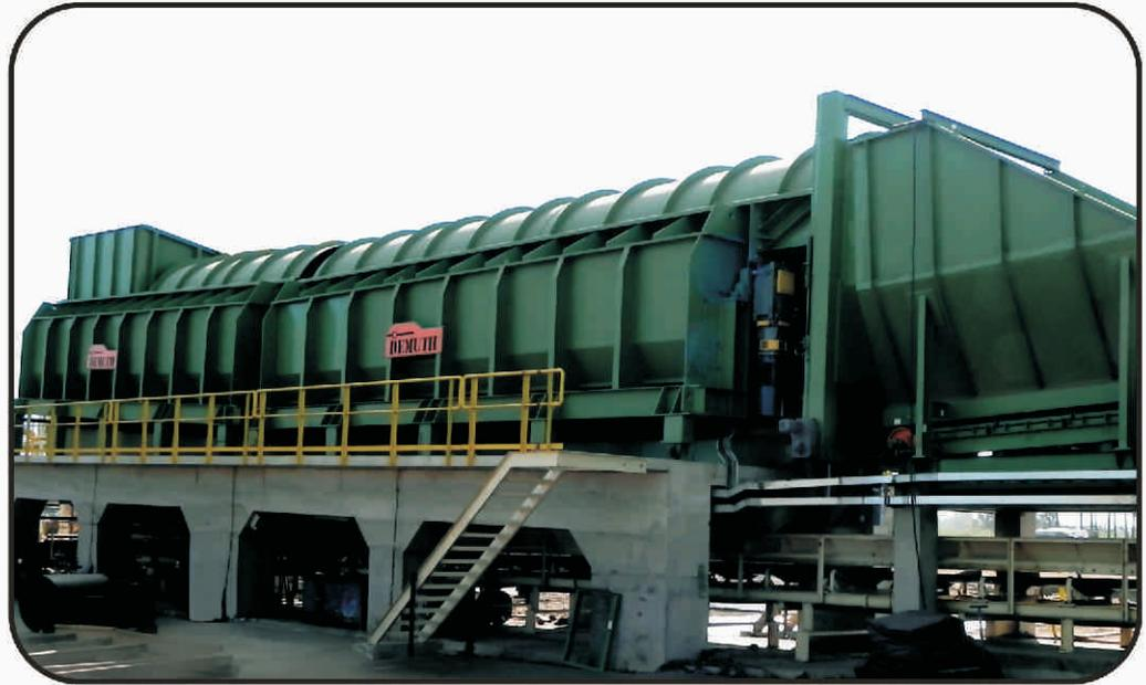
Each debarking module is built with three rollers, made of sturdy industrial tubes, with heavy duty shafts and special over dimensioned house bearings. The rollers are provided with replaceable abradars, made of high wearing resistance material.
