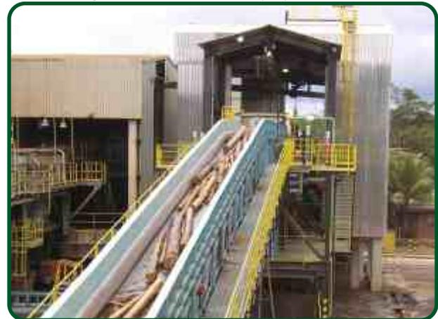
Located in Belo Oriente/ MG, the project consists in a chipping line with nominal capacity for 250m<sup>3</sup> sub/h. Main line equipment are a Feeding Table (Master Feed), a DPVD 3000 disc chipper and a DPO 900 chip screen.
