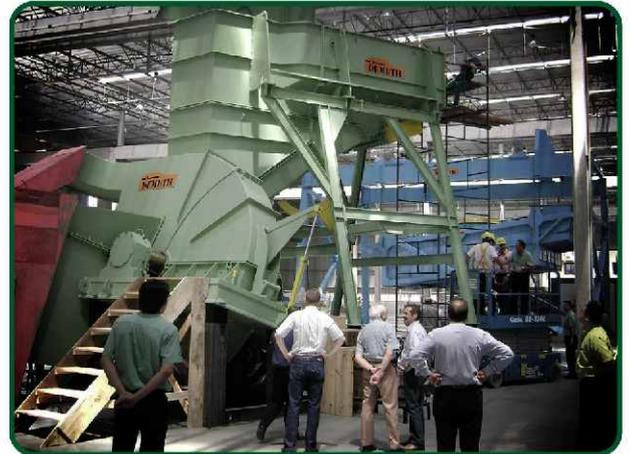
*A modern and simple design provides a high availability rate, easy operation and maintenance. Chipper idealized to process long and short logs, with high flexibility to be adjusted to different chip dimensions. The chipped material outlet can be downwards, by gravity or backwards, onto a flow equalizing bin and screw or by a belt conveyor.*
