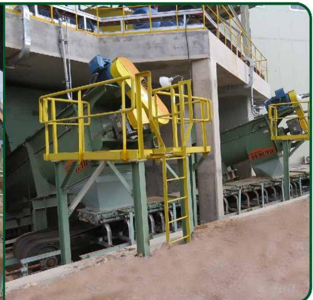
Equalizing Screw / Rosca Dosadora de Cavacos
