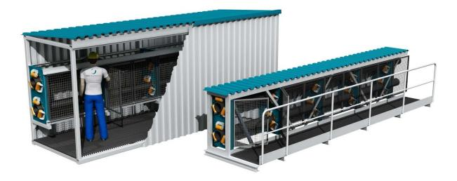
Tubular belt conveyors are a good choice for conveying various kinds of bulk materials over long distances at high capacities. The material lies unaffected on the conveyor belt throughout its journey between the transfer points.
