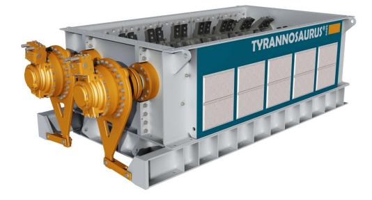
TYRANNOSAURUS<sup>®</sup> 6600 Preshredders are the best solution available on the market for rough shredding of material during pre-treatment. They are designed to open e.g. plastic bags and crush the MSW (Municipal Solid Waste) into a smaller particle size which then allows proper separation in the drum screen. TYRANNOSAURUS<sup>®</sup> 6600 Preshredders can also operate as the main shredder for grate fired incinerators.
