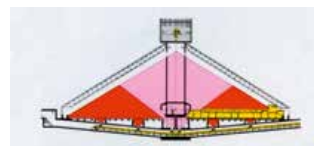
Covered stockpile with MOLEX® and central column
