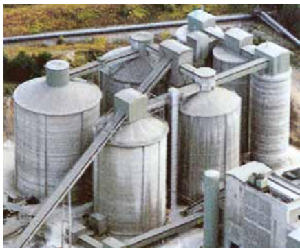
Silo group for different clinker types
