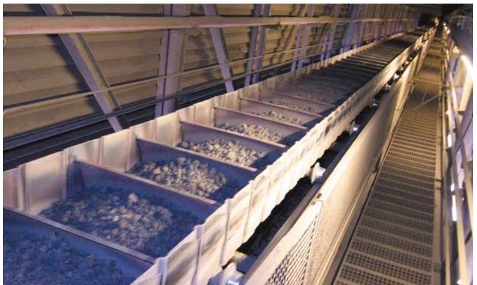
KZB-Q inclined at 45 degrees
