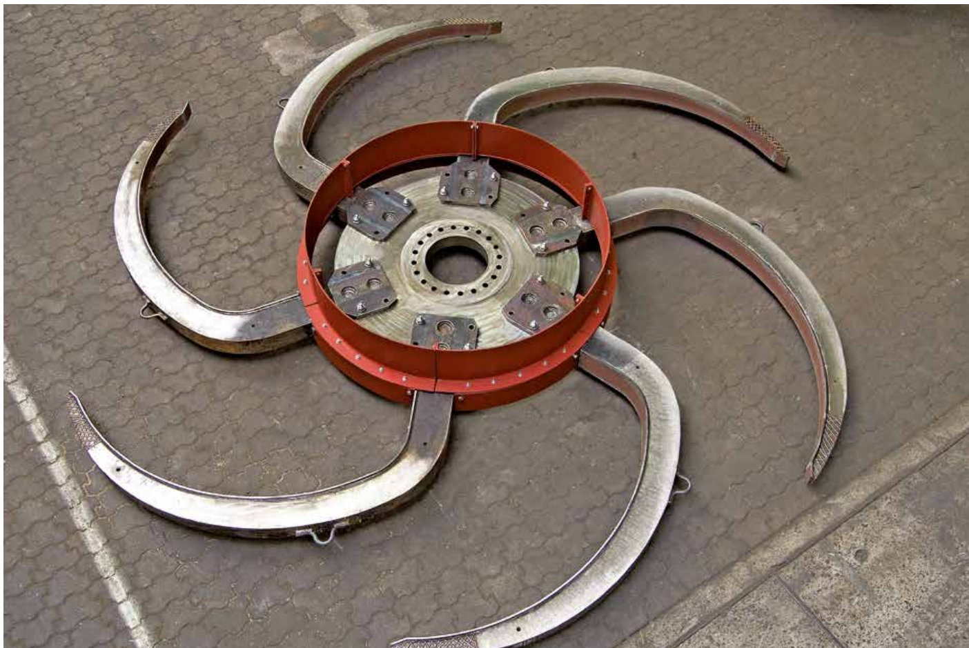
BEW-K discharge wheel, \varnothing 4,500 mm
