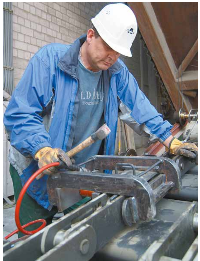
Pre-assembly of chain strands
