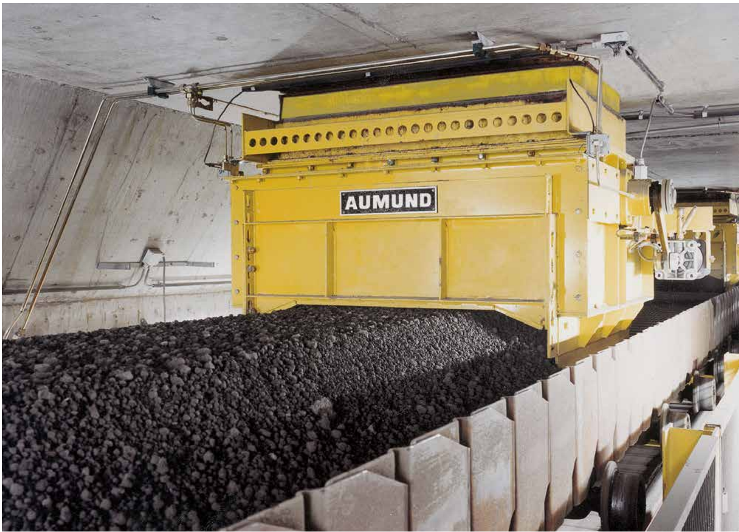
Silo Discharge with Remote Control
