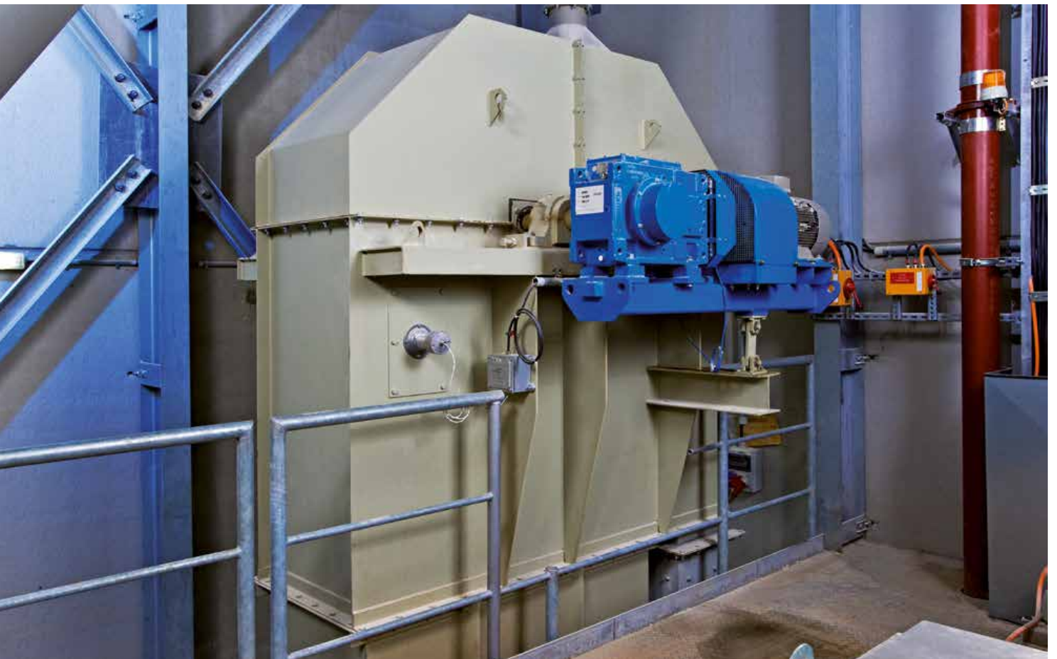
Bucket elevator head with single drive
