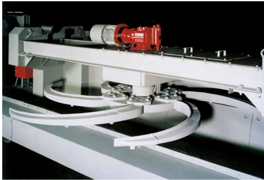
View onto discharge wheel
