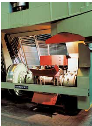
Internal ring with thrust bearings and travel unit
