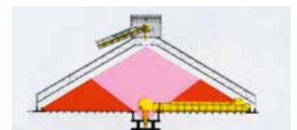
Covered stockpile with MOLEX® without central column
