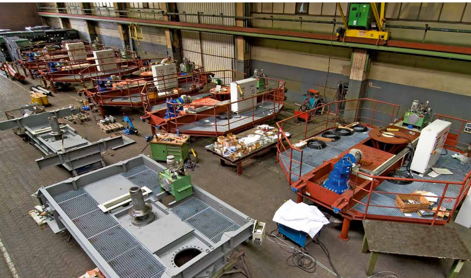
5 BEW-K's 10,000/4,500 during assembly in the workshop
