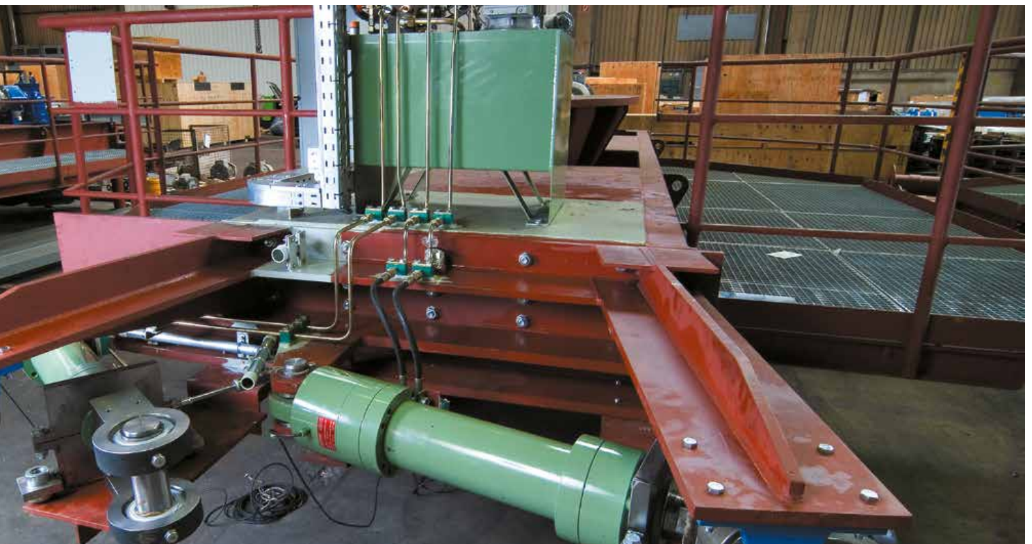
Chassis of BEW-K, view onto hydraulic cylinders for rotation
