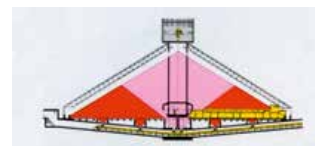
Covered stockpile with MOLEX® and central column
