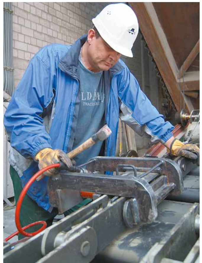
Pre-assembly of chain strands
