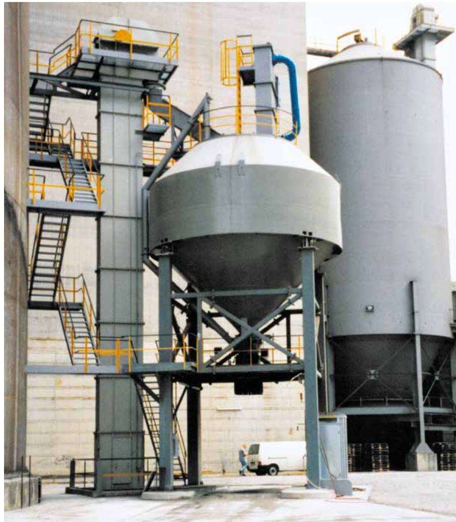
Bucket Elevator for low to medium capacities
