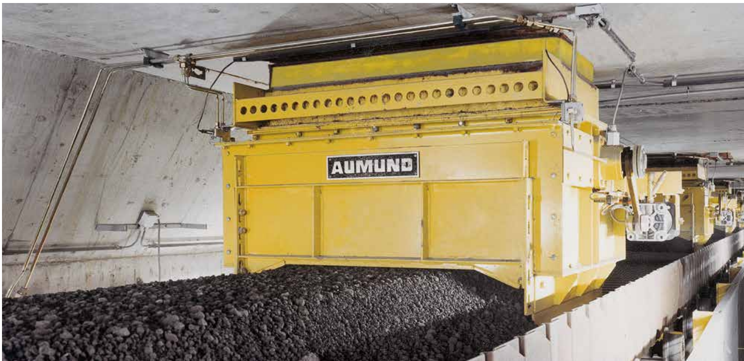
Silo discharge by remote control – discharge capacity 750 t/h
