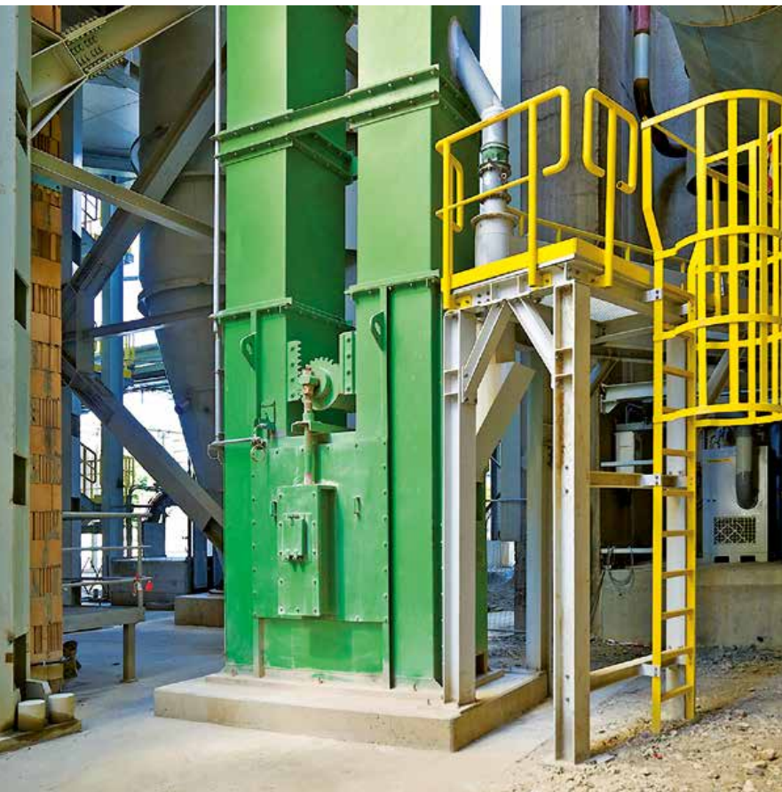
Elevator boot with parallel tensioning device
