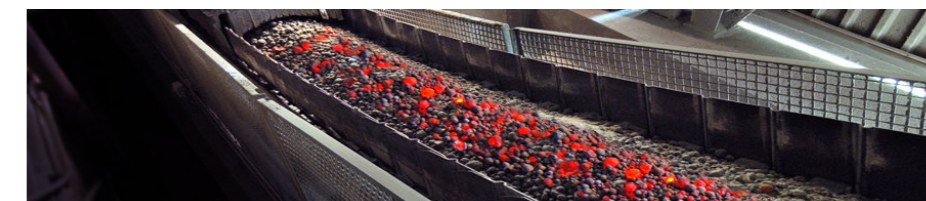
Pivoting Pan Conveyor (SPB)
