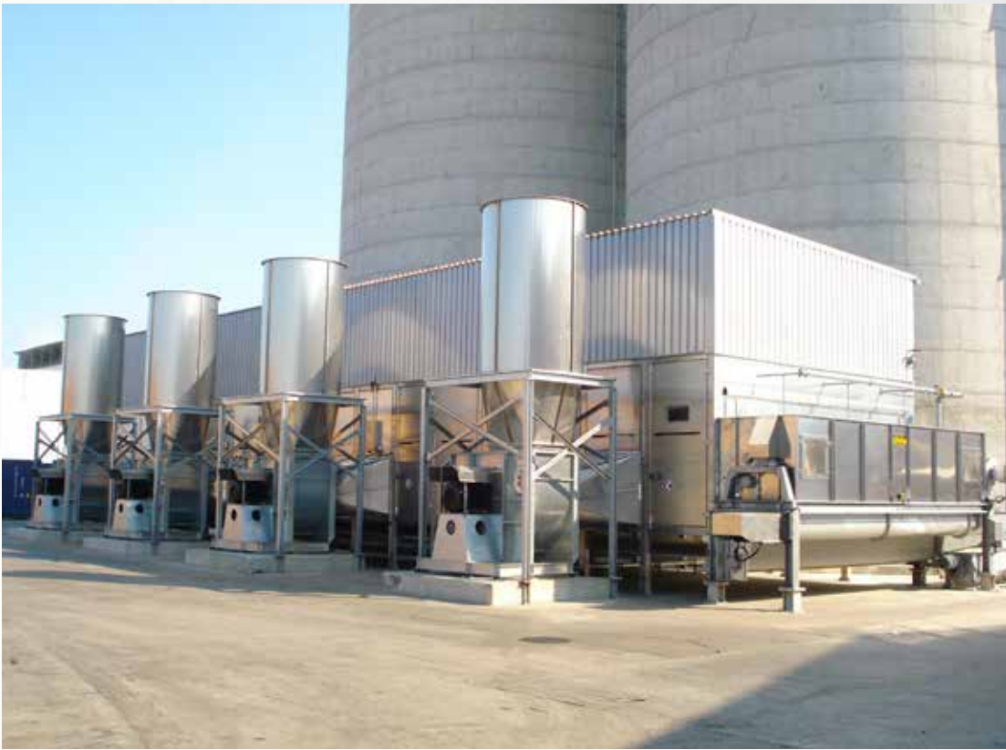
Project: Schweighofer Rumania, Sebes Type: BT 1/6200-25,5 Year: 2007 Product: sawdust Dryer output capacity: 8,0 t/h from 50% - 10%
