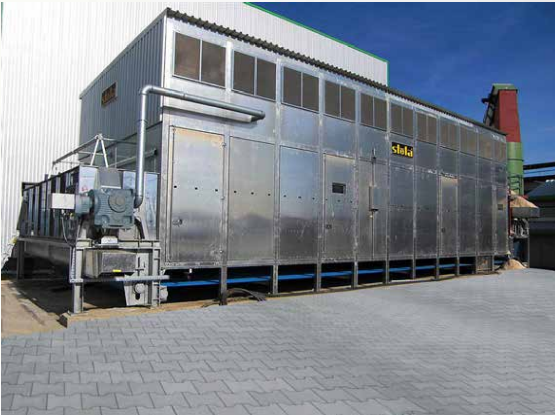
Project: Ameco Rumania, Gheorgheni Type: BT 1/6200-16,5 Year: 2009 Product: sawdust Dryer output capacity: 6,0 t/h from 50% - 10%
