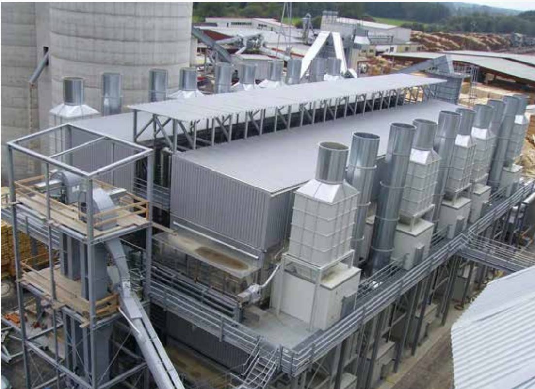
Project: Pfeifer Holz GmbH Germany, Unterbernbach Type: 4x BT 1/6200-36 Year: 2007 Product: sawdust Dryer output capacity: 50,0 t/h from 50% - 3%
