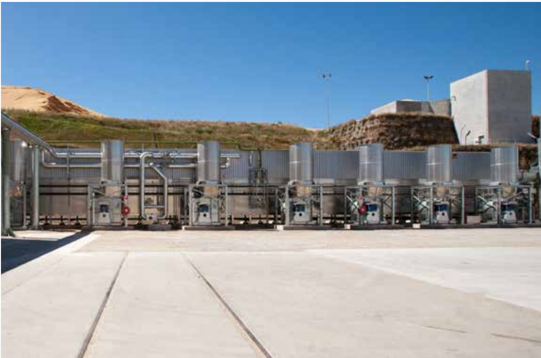
Project: Nature's Flame New Zealand, Taupo Type: BT 1/6200-52,5 Year: 2009 Product: sawdust Dryer output capacity: 12,0 t/h from 60% - 10%
