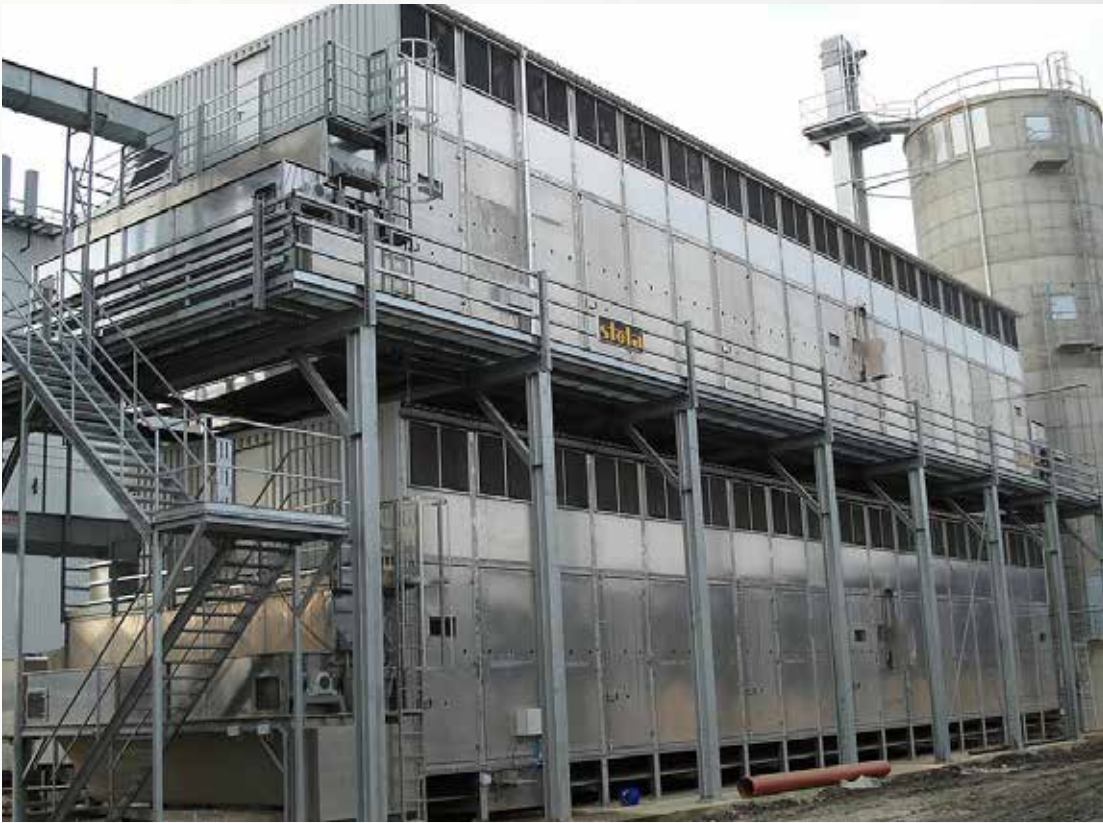
Project: ERDA Belgium, Bertrix Type: 2x BT 1/6200-27 Year: 2006 Product: sawdust Dryer output capacity: per 16,0 t/h from 50% - 10%
