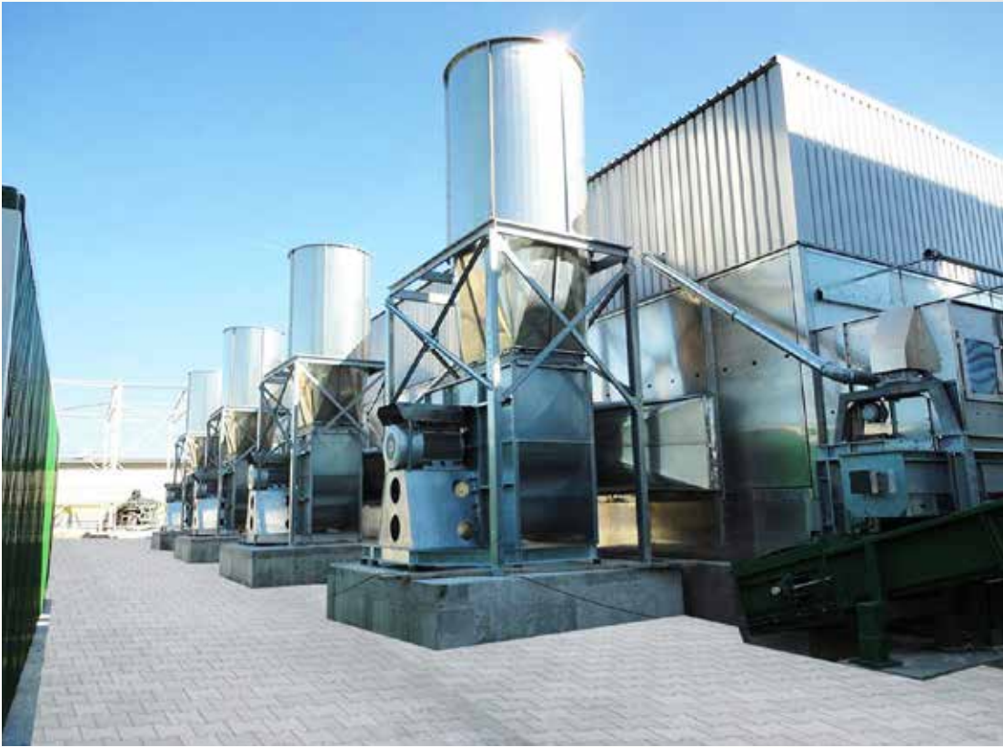
Project: Hekotek Estonia, Jüri Type: BT 1/6200-34,5 Year: 2011 Product: sawdust Dryer output capacity: 12,0 t/h from 53% - 11%
