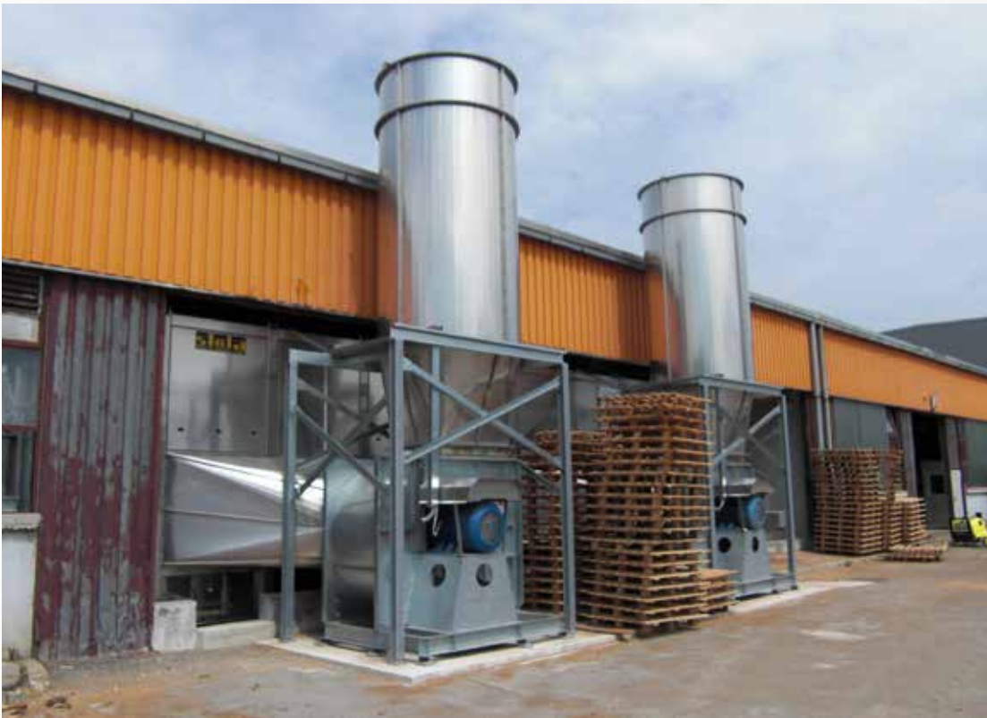
Project: Moderator d.o.o Croatia, Udbina Type: BT 1/6200-13,5 Year: 2011 Product: sawdust Dryer output capacity: 5,0 t/h from 45% - 10%
