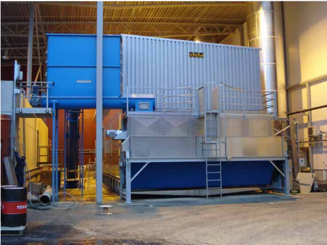
Project: Torkapparater Sweden, Stockholm Type: BT 1/6200-19,5 Year: 2009 Product: sawdust Dryer output capacity: 12,2 t/h from 50% - 26%
