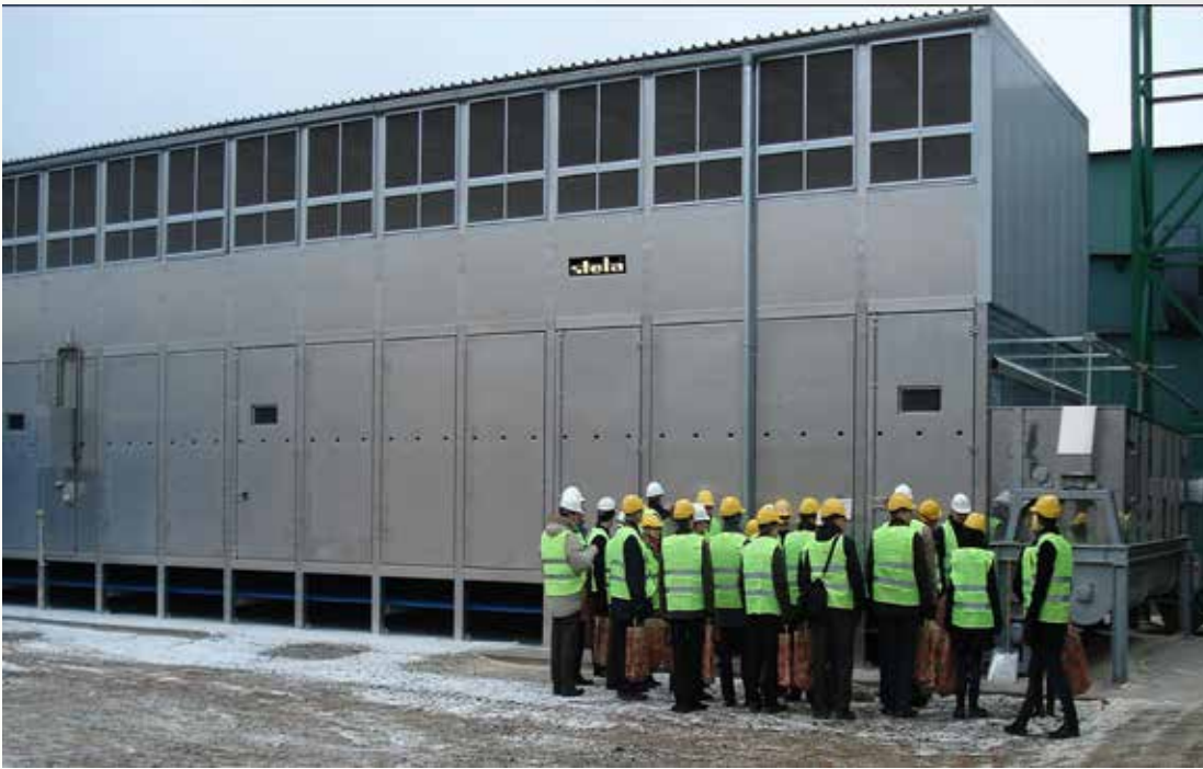
Project: Stora Enso Timber Sweden, Grums Type: BT 1/6200-36 Year: 2008 Product: sawdust Dryer output capacity: 10,0 t/h from 52% - 10%
