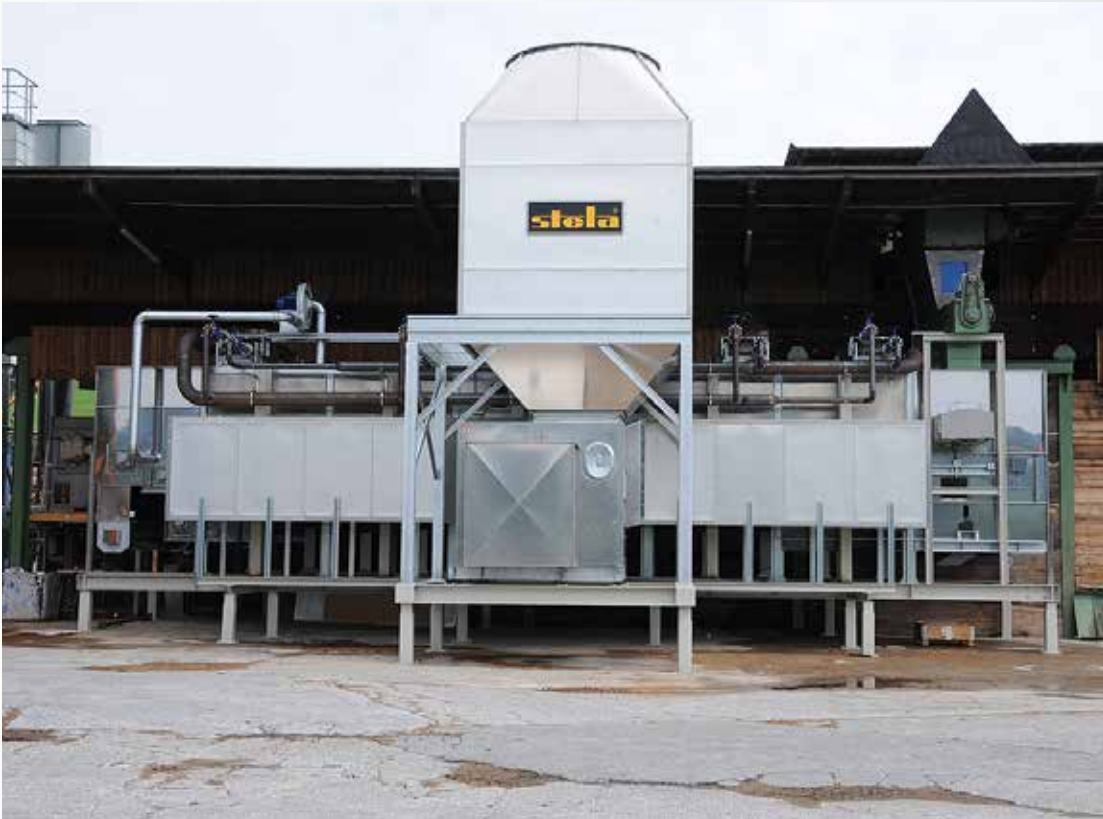
Project: Baust Holzbetriebe Germany, Eslohe-Bremke Type: BT 1/2700-11 Year: 2010 Product: sawdust Dryer output capacity: 1,6 t/h from 50% - 10%
