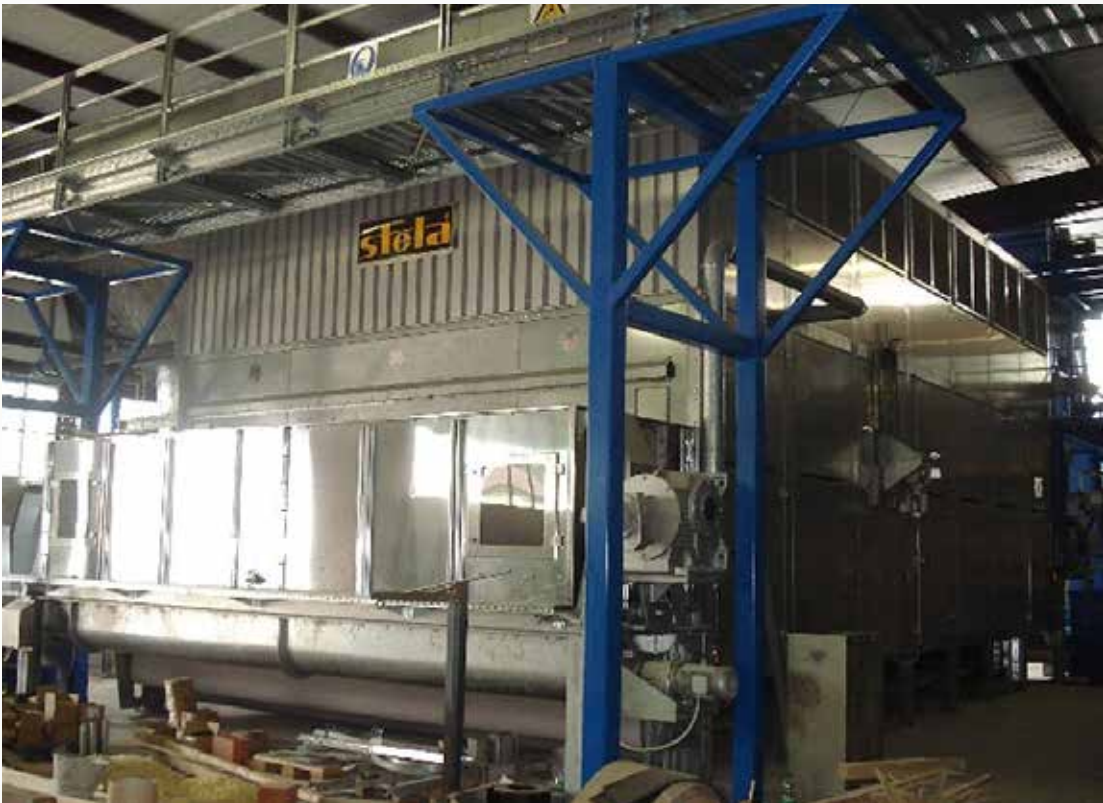
Project: Finvest Croatia, Gerovo Type: BT 1/6200-10,5 Year: 2007 Product: sawdust Dryer output capacity: 3,6 t/h from 50% - 13%
