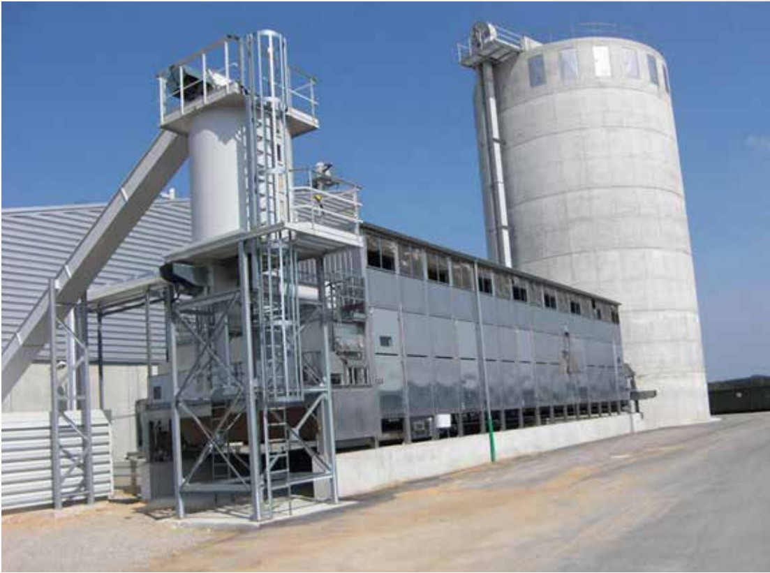
Project: Pröbstl Germany, Fuchstal Type: BT 1/6200-22,5 Year: 2007 Product: sawdust Dryer output capacity: 8,0 t/h from 50% - 10%
